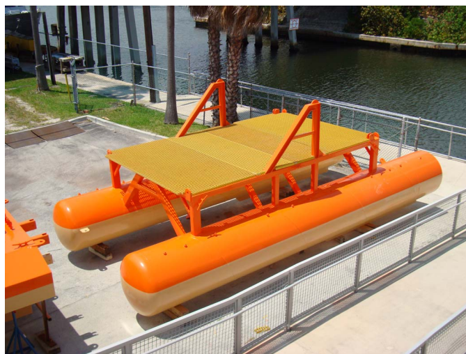
Figure 3. The complete OCDP without A-frame, hydraulic, and electronic systems.
